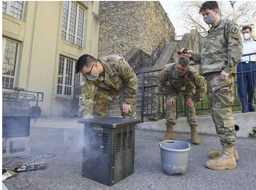
Cadets Stephen Moryl '21, Dan Carlson '21, and Calvin Fuller '21 test their dung-burning stove outside Nichols Engineering Building March 26, under the supervision of Maj. Morgan Bruns.—VMI Photo by H. Lockwood McLaughlin.
