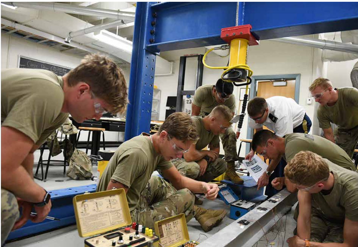
Cadets in Col. Matt Swenty's civil engineering lab set up gauges before stress testing an aluminum I-beam.—VMI Photo by Mary Price.
