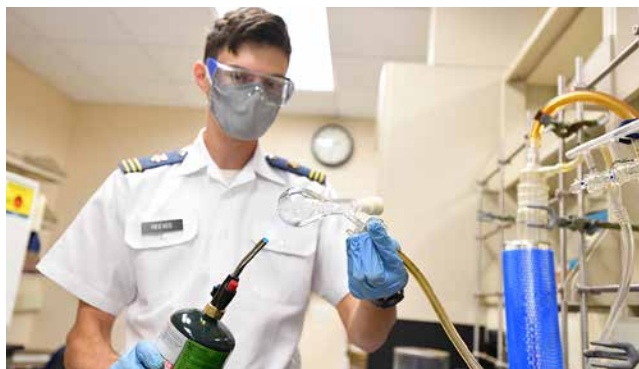
Kellen Reeves '21 flame dries a flask before performing a water-sensitive reaction.—VMI Photo by Kelly Nye.
